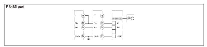
RS485 NOTE: additional devices provided with RS485 are connected as per the picture above. The termination of the serial output is carried out only on the last instrument of the network, by means of a jumper between (B+) and (T).
