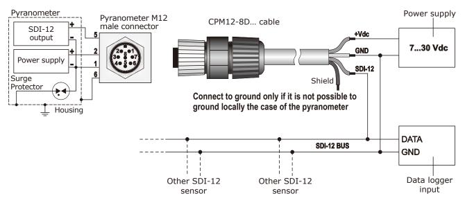
Fig. 4.5: LPPYRA10S12 connections
