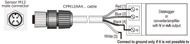
ground locally the case of the pyranometer
