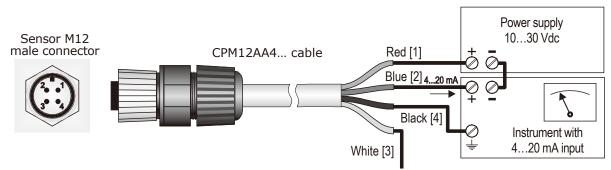
Connect to ground only if it is not possible to ground locally the case of the pyranometer
