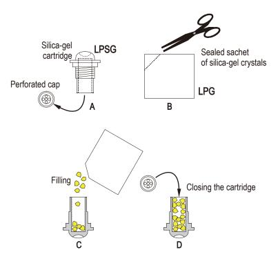
Fig. 3.1: filling the silica-gel cartridge
