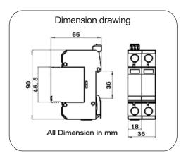
Type 2 surge arrester designed for low voltage DC system against surges at the boundaries from lightning protection zone OB-2and higher.
