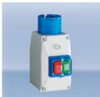
Insulated enclosure with IP54 SCHUKO earthed plug with 2 earthing systems acc. to CEE7/II 16 A 250 V, 2-pole + ⊕ 1 opening at the bottom
