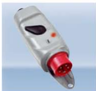
CEE ON/OFF switch ML0 - Plug 32A 5p 400V with phase inverter
