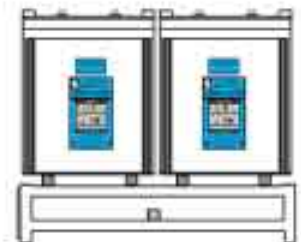
Typical standard rack for vertical cell configuration
