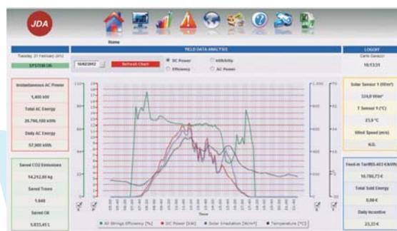
The causes of inefficiencies can be located in either DC generation or DC/AC conversion (inverter) area, therefore a very powerful analysis tool is needed. The combined DC power, DC current, DC voltage and solar irradiation answers to the DC generation question, it provides all the information which are needed to localise the problem.
