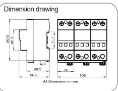
DC SPD designed for low voltage system protection against surges at the boundaries from lightning protection zone 1-2 and higher.
