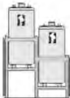
Typical anti-seismic rack for vertical cell configuration of SEC-OPzV range of batteries
