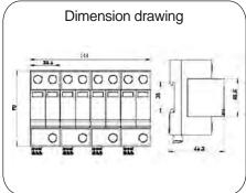
Type 1 CA surge protective device is especially designed for low-voltage power supply system at the boundaries from lightning protection zone 1-2 and higher.
