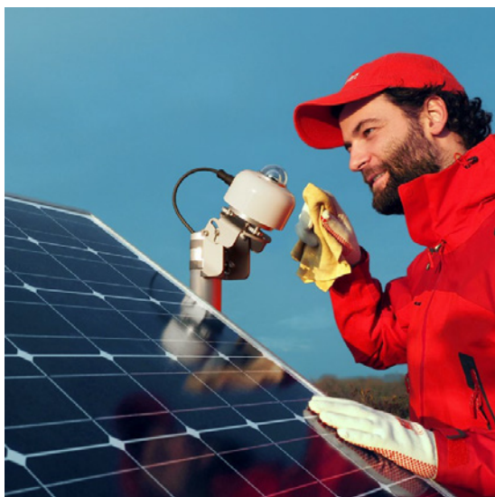
Figure 2 SR15-A1 pyranometer mounted in POA (Plane Of Array) on a mast for PV performance monitoring
