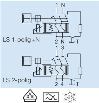
RCBOs offer a compact possibility of implementing wiring protection and protection against personal injury in one device. The RCBO protects itself through its CB part against overload. An undesired overload due to too-high load currents is not possible. One RCBO is assigned to every circuit. So the full fault current is available to every circuit as drainage current. For one fault current in a circuit, only the affected circuit is switched off.
