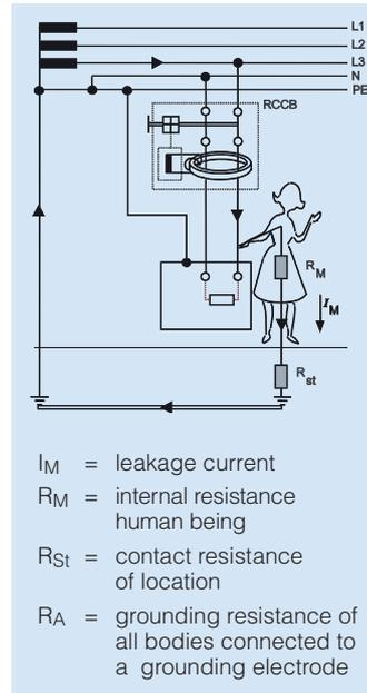
**Fire protection according to DIN VDE 0100-482**
