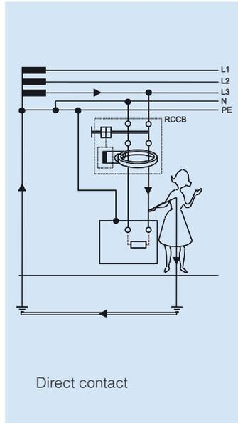
**Protection against leakage currents according to DIN VDE 0100 Part 410**
