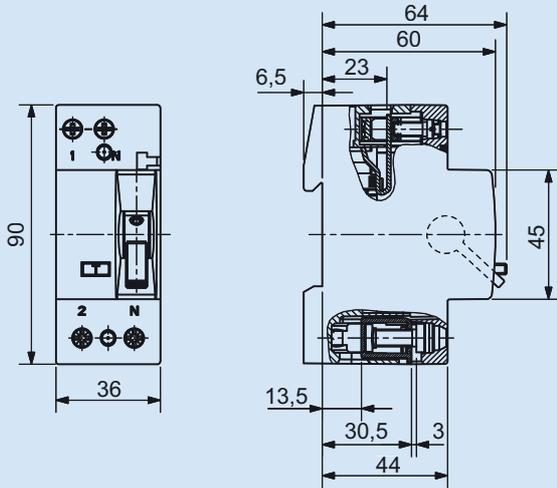
**Auxiliary contact for 2-pole and 4-pole RCCBs 16 up to 80 A,
