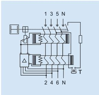
RCCBs of type B, as well as detecting residual current shapes of type A, are also used for detecting smooth DC residual currents and for input circuits 7 to 10 according to table "Technical Data – fault current forms" (see left page).
