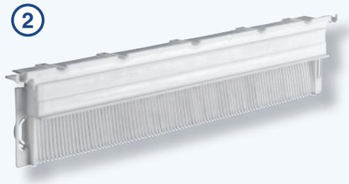
Patented self-latching sliding section with automatically retractable comb pins. No need to break or cut out cable glands; wiring can be easily installed.
