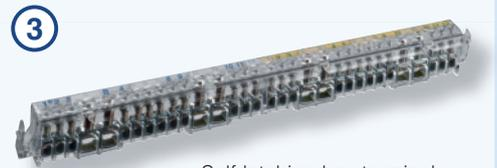
Self-latching box terminal strip for wire connection up to 25 mm<sup>2</sup> (in) and 10 mm<sup>2</sup> (out). Finger safe according to BGV A2 (VGB 4). Screws are open for shipping and cannot be lost.
