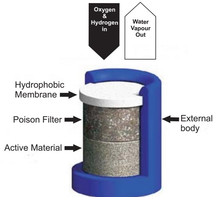
Today, SEC has extensive experience of the benefits of using Catalysts in our sealed VRLA cells, and we offer Catalyst equipped products in our 2 volt and 6-12 volt Monobloc batteries. We are also continuing our research and development program into new alternative Catalyst technologies and will be launching further new products in this area in future.
