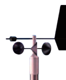
風速&風向計 Wind speed and direction
