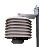
温度&湿度情報発信機 Outdoor temperature and humidity transmitter
