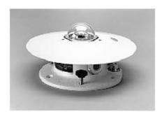
There are two generally accepted Classification Systems used for Pyranometers. ISO classifies pyranometers as a "Secondary Standards", "First Class" or "Second Class" while WMO uses "High Quality", "Good Quality" and "Moderate Quality".
