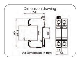
Type 2 surge arrester designed for low voltage DC system against surges at the boundaries from lightning protection zone 0B-2and higher.
