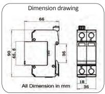
Type 2 SPD designed for low voltage system protection against surges at the boundaries from lightning protection zone 1-2 and higher.
