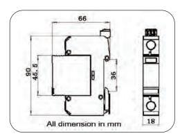
Type 2 AC surge arrester designed for low-voltage power supply system protection against surges at the boundaries from lightning protection zone 1-2 and higher.
