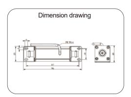
JDA DN-24/BNC-50 surge arrester is designed for coaxial systems protection against the damaging from surges and spikes caused by lightning and other electrical sources, suitable for use in category location B, C (ANSI/IEEE C62.41) or directly at the upstream near the protected devices.
