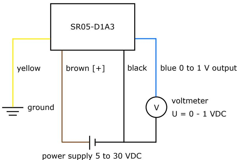
**Figure 5.8.1** Electrical diagram of the connection of SR05-D1A3 to a typical voltmeter or datalogger with the capacity to measure voltage signals. SR05-D1A3 operates on a supply voltage of 5 to 30 VDC.
