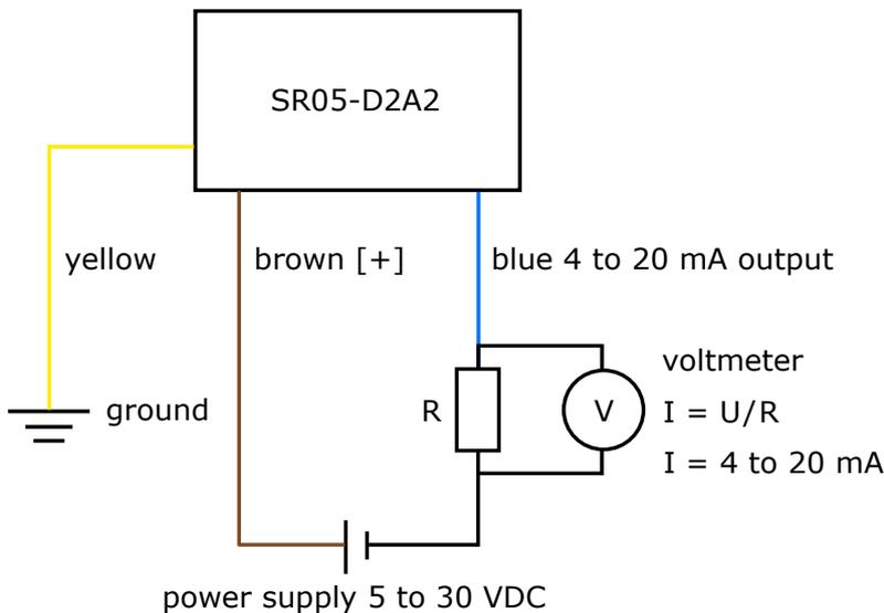
**Figure 5.9.2** Electrical diagram of the connection of SR05-D2A2 to a typical voltmeter or datalogger with the capacity to measure voltage signals. Usually a 100 Ω shunt resistor (R) is used to convert the current to a voltage. SR05-D2A2 operates on a supply voltage of 5 to 30 VDC.
