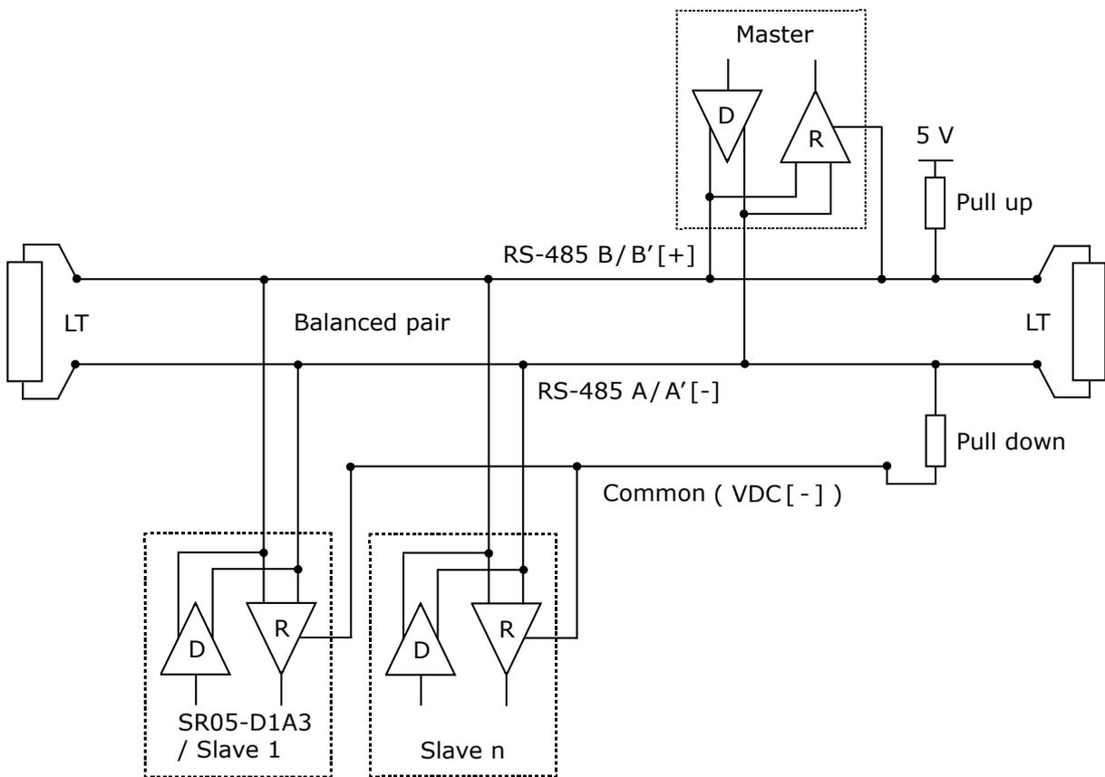
**Figure 5.11.1** Typical topology of a two-wire RS-485 network, figure adapted from: *Modbus over serial line specification and implementation guide V1.02 (www.modbus.org)*. The power supply is not shown in this figure.
