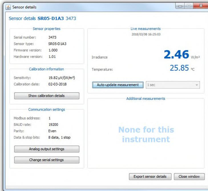
**Figure 6.1.5.1** Sensor details window in the Sensor Manager
