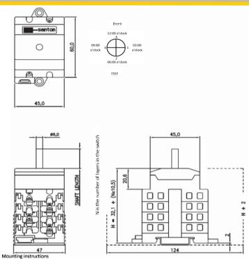
In the application all ratings have to be respected. When building the switch in an enclosure, the space envelope must be respected according to the applicable standards. After mounting, the wiring must be checked and the switch must operate smoothly.
