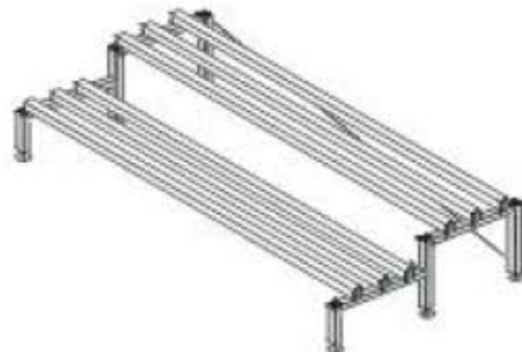
Typical standard rack for vertical configuration of SEC OPzV range of batteries
