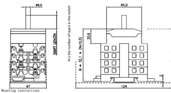
In the application all ratings according to the datasheet have to be respected. After mounting, the wiring must be checked and the switch must operate smoothly. When building the switch in an enclosure, the space envelope must be respected according to the applicable standards.
