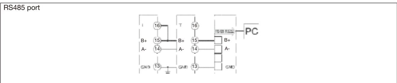
RS485 NOTE: additional devices provided with RS485 are connected as per the picture above. The termination of the serial output is carried out only on the last instrument of the network, by means of a jumper between (B+) and (T).
