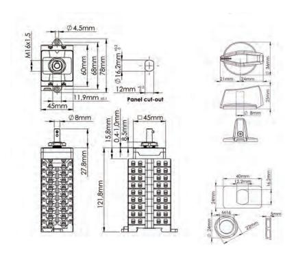
The tolerances for the Santon datasheet are according to ISO 1101, ISO 8015, ISO 2768 1 class m, unless stated otherwise.
