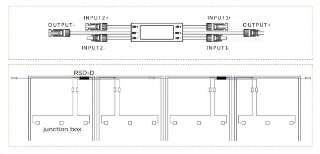
RSD-D can be installed together with RSD-S-PLC;
