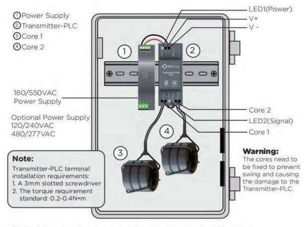
Note: If there is only one core needed, connect using Core 1 terminal.
