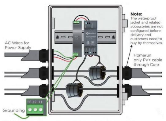
**Note:** 180/550Vac power supply isolation class I requires grounding. 85/264Vac power supply isolation class II does not require grounding.
