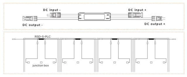
**NOTE:** Do not short-circuit the RSD-S-PLC output connectors, otherwise it will be damaged.
