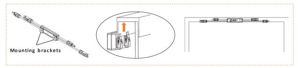
**NOTE:** Do not place the RSD (including DC connectors) where exposed to the sun, rain or snow, even gap between modules. Any surface of the RSD other than the mounting bracket must be at least 15mm away from surrounding objects. In particular, it is forbidden to have DC cables run close to or cover the RSD casing.
